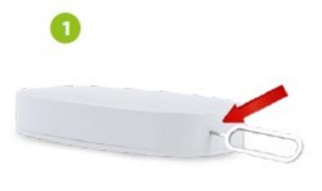
Using the PIN included, press and hold the RESET button for 8 seconds until the green LED starts flashing.
