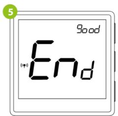
6. Both devices have been successfully linked. The thermostat displays the main screen, the icon " ((中)) " appears on the screen indicating connection with the receiver (ECB62ZB in this case).
