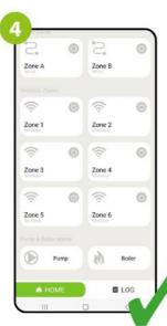
The control box has been installed and displays the main interface. Power diode lights up blue.
