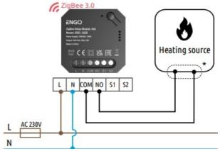
• b) Connection diagram for pump / actuator
