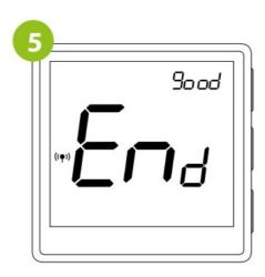
After successfull binding operation "End" message will be displayed. LED on the module will stop flashing.
