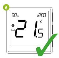
Both devices have been successfully linked. Thermostat displays the main screen, icon " <sup>((</sup>)" appeared on the screen indicating connection with the receiver (ECB62ZB in this case).
