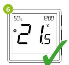
On the controller screen globe icon appeared stating that he has been he added to the ZigBee network.
