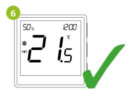
Both devices have been successfully linked. Thermostat displays the main screen, icon " ((๑))" appeared on the screen indicating connection with the receiver (module/relay in this case).
