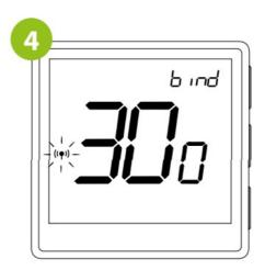
The "binding" process takes up to 300 seconds.
