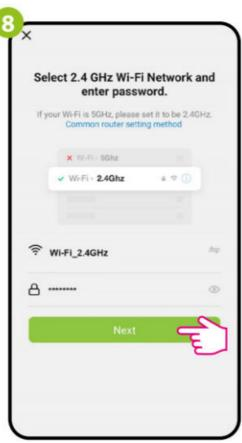
Select the Wi-Fi network in which the gateway will operate and enter the password of this network.
