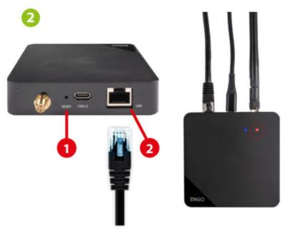
Make sure the device is connected to the power supply and to the Internet via the cable (2).
