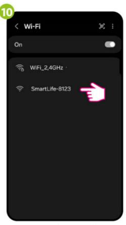
The device will go to the Wi-Fi network settings screen. Select the "SmartLife-XXXX" network and connect to it.
