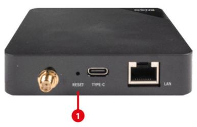
To restore the default settings of the device, press the RESET button (1) and hold it for approx. 10 seconds – until both LEDs light up. Then release the button, the universal internet gateway will restore the default (factory) values and the pairing process will begin.
