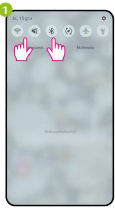
On the mobile device, make sure that the ENGO Smart app has access to the permissions (Location, Bluetooth, Nearby devices). Then turn on Bluetooth and location. Connect tothat 2.4 GHz Wi-Fi network to which you want to assign the gateway (Wi-Fi and wired Ethernet must be one network – from the same router).
