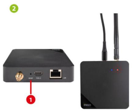
Make sure the unit is powered on. Then press and hold the RESET button (1) (using the pin provided) for 10 seconds. The red LED must flash slowly, then the gateway is in pairing mode.
