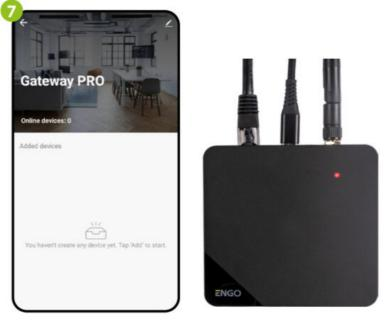
The gateway has been installed and displays the main interface. On the device, the red LED lights up continuously.
