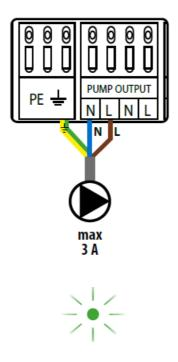
When the Pump/Valve control output is activated, the pump status LED shows a constant green light.
