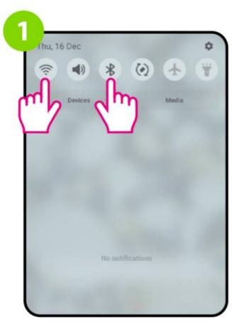
On your mobile device, make sure the ENGO Smart has access to permissions (Location, Bluetooth, Nearby devices). Then turn on Bluetooth and Location. Connect to 2.4GHz Wi-Fi network to which you want to assign the device.
