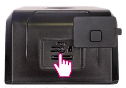
Make sure the camera is powered on. Then press and hold the button on the back of the camera for approximately 5 seconds, until the beep. The blue LED on the front of the unit will then start flashing. The pairing mode is enabled.
