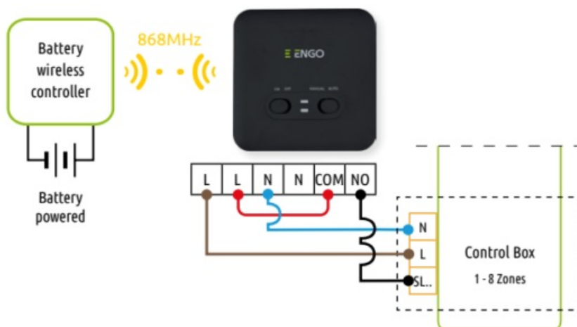
c) Connection diagram of receiver to control box
