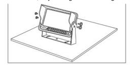
2) U-Bracket Installation (optional) 1) Use the screw fixed the U-bracket. Put the monitor into the bracket, adjust angle and locking it.
