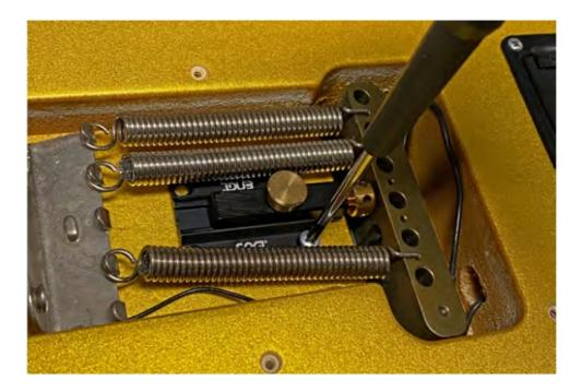
5. Mark the remaining holes, drill and finish assembling the Hardtailer. Remove springs if necessary.
