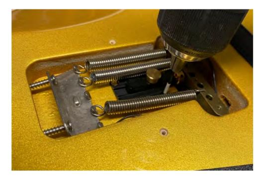
4. Screw tight the Hardtailer with included screws.
