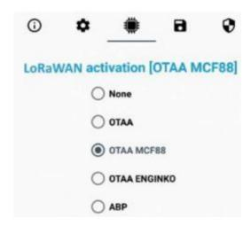
The device exits factory activated with NONE mode. On request devices can be shipped aleady activated. **Note:** in OTAA AppKey is write only, in reading the field will always be empty, even if set.
