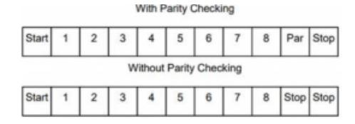
Even parity is required, other modes (odd parity, no parity) may also be used. In order to ensure a maximum compatibility with other products, it is recommended to support also No parity mode. The default parity mode must be even parity. Remark: the use of no parity requires 2 stop bits.
