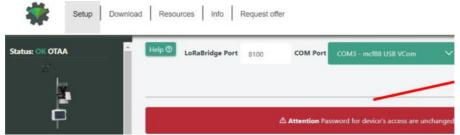
To bring back the sensor to factory default and reset the passwords, a reset code must be requested to enginko (please provide the DevEUI of the sensor when you ask for that code).
