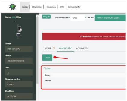
Press Check to verify the correct communication betweet the LoRaWAN® interface and the slave(s).
