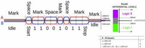
The objective of biasing is to make sure that the RS485 line remains in a known, non-fluctuating state when no devices are transmitting. Polarization of the pair must be implemented at one location for the whole serial bus.
