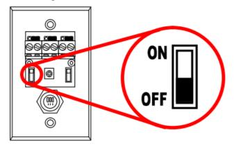
**ON:** LED is green while in standby and turns red when triggered.
