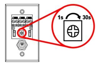
Output duration is adjustable 1~30 seconds. (Must be set to 'Timer' in step 4)
