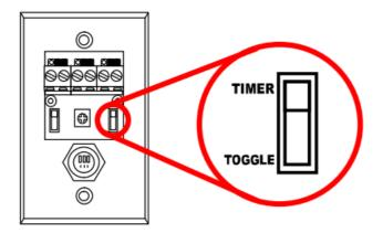
**TIMER:** When set to TIMER, pressing the switch will trigger the relay for the set duration. Set the time using the trimpot as described below.
