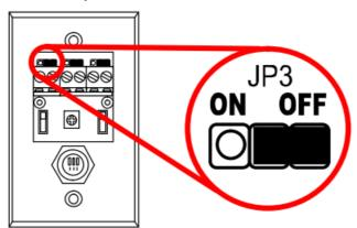
Use the buzzer output jumper JP3 to program the buzzer output. Placing the jumper on the left turns the buzzer output ON. Placing the jumper on the right turns the buzzer output OFF.
