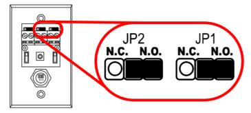
Outputs 1 and 2 can be set independently using jumpers JP1 and JP2. Note: Both outputs trigger simultaneously. Place the jumper on the right for N.O. operation and on the left for N.C. operation.
