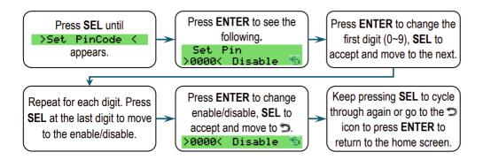
If you forget the PIN Code, proceed as follows to unlock the timer and enter programming mode.
