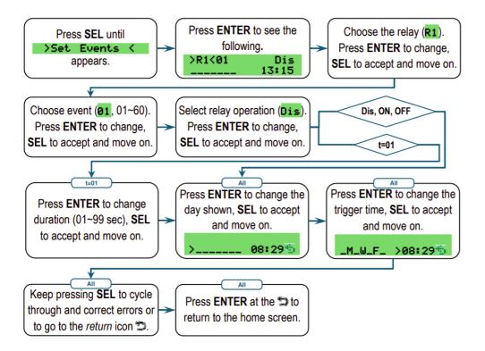
**NOTE**: Relay operations are Dis (shunt), ON, t=x (momentary, where x=01~99 seconds), or OFF.
