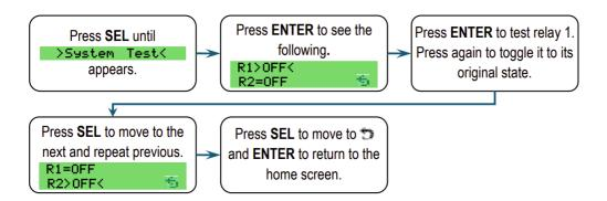
**NOTE:** Performing the system test on a relay toggles that relay based on its current state. If the relay is currently ON, pressing ENTER to test will toggle it OFF and vice versa. If currently OFF, it would toggle to ON.
