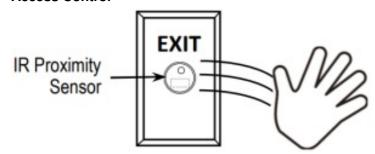
• Mount the sensor to a wall or plate in a protected area. A user can wave his or her hand in front of the sensor to unlock an electronic door lock, allowing germ-free, protected egress
