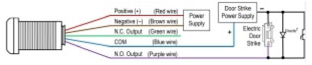
†Suggest connecting a metal oxide varistor (MOV) and diode (both not included) as close as possible and in parallel with the controlled output
