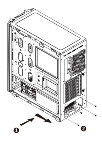
Move to HDD cage forward to create extra space for a 200 mm  $\mbox{PSU}$
