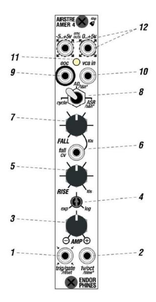
1. TRIG / GATE / RESET JACK INPUT: multifunctional pulse input.
