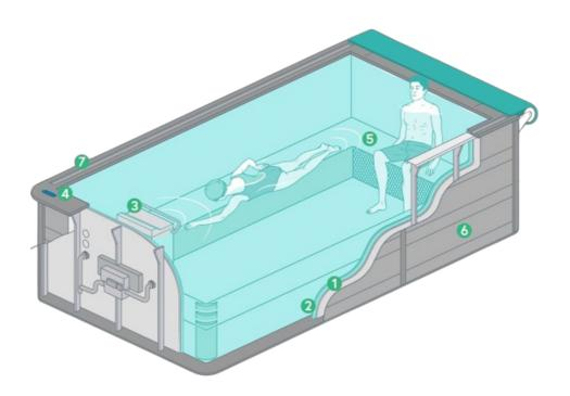
Sturdy and rust-resistant, our 14-gauge galvanized steel panels give you the flexibility to adjust your pool's size in one-foot increments. These panels come with a 10-year structural warranty.
