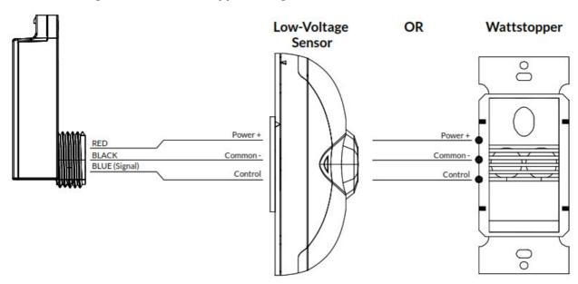
2. SIM to Sensor Junction Box Wiring
