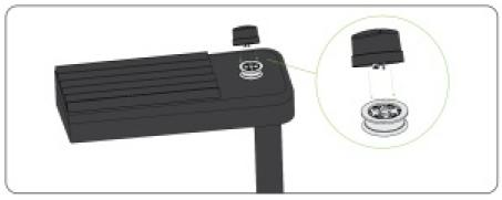
2. Mount the control with the arrow and 'N' on the cover facing north.
