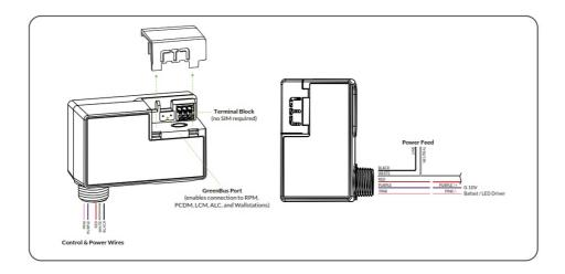
Recommended branch circuit, 120-347V, 20A maximum. Recommended dimming signal capacity, 0-10V, 30mA maximum (sinking).
