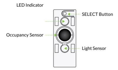
DALI LS PD LI features an Occupancy and Light Sensors, SELECT Button, and LED Indicator. The SELECT Button enables you to identify a device and reset to factory default settings. The LED Indicator displays green or red lights (see the DALI LS PD LI LED Indicator details below).
