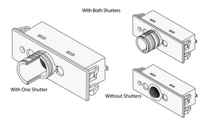
The detection range of the DALI LS PD LI sensor is determined by the shutter position.
