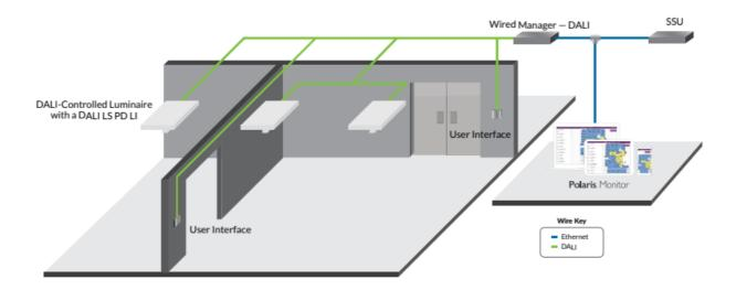
Encelium X enables you to control DALI devices. With any Encelium wired design, you get a reliable, lighting control system that can be installed quickly and easily.
