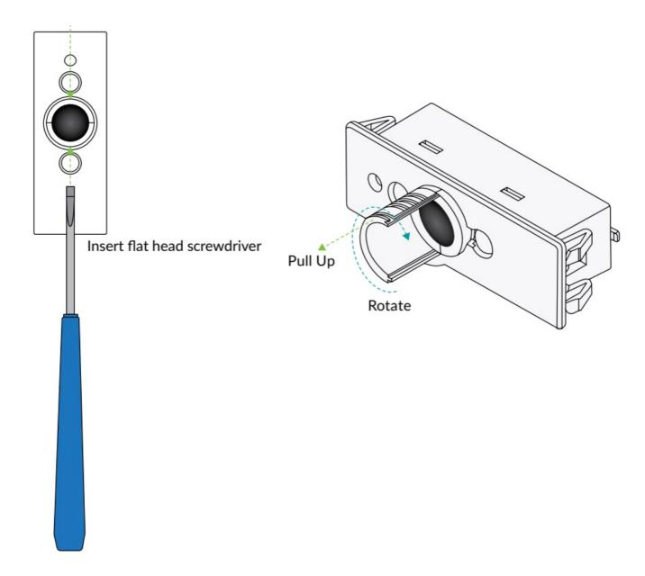
Using a small screwdriver pull up on the shutter sides. Remove, insert, or rotate one or both shutters where necessary.
