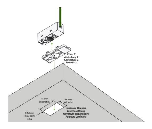
A 14 x 41 mm (0.5 x 1.6 inches) hole must be cut prior to installing the DALI LS PD LI. Install Cover 2 on the DALI LS PD LI and connect the sensor cable to the DALI Line. Then place the DALI LS PD LI into the luminaire hole. Secure the DALI LS PD LI by snapping the cover mounting clips into the luminaire. The raised surface of the cover sits flush within the luminaire opening.
