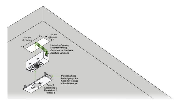
A 15.4 x 55.4 mm ( $0.6 \times 2.2$  inches) hole must be cut prior to installing the DALI LS PD LI. Install Cover 1 on the DALI LS PD LI and connect the sensor cable to the DALI Line. Then place the DALI LS PD LI into the luminaire hole. Secure the DALI LS PD LI by snapping the cover mounting clips into the luminaire. The raised surface of the cover sits outside the luminaire opening.
