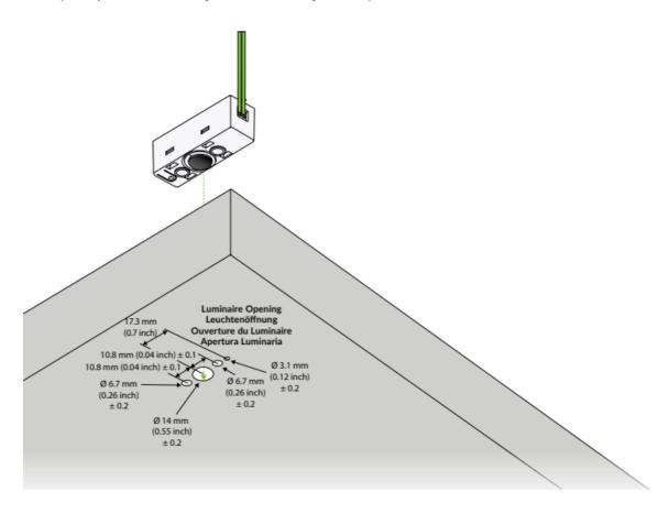
Holes must be cut prior to installing the DALI LS PD LI. Connect the DALI LS PD LI sensor cable to the DALI Line. Then place the DALI LS PD LI into the luminaire holes. If the sensor is in the correct mounting position, the raised surface of the sensor sits flush within the luminaire opening.
