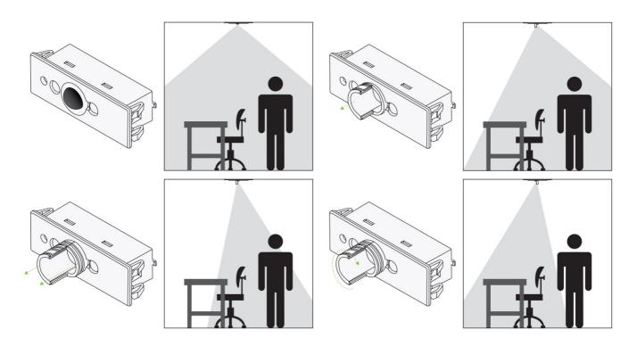
By changing the shutter position, you can influence the detection range of the sensor directionally and avoid undesired presence detection.
