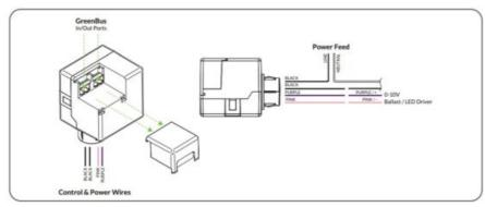
**Notes:** Recommended Relay switching capacity, 120–347V, 20A maximum. Recommended Dimming signal capacity, 0-10V, 30mA maximum (sinking).
