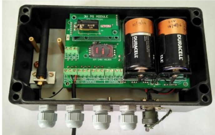
Figure 4-1 Datalogger powered with 2 x 1.5 V Alkaline Batteries
