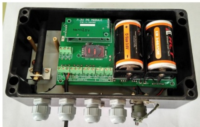
Figure 4-2 Datalogger powered with 2 x 3.6 V Lithium Batteries
