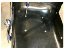
If necessary, you can straighten the plate or rants with a set of vice grips. If you are still having difficulty, the holes in the Repair Channel can be drilled out to the next size up.
