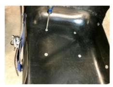
3. Unfasten the two 1/4-20 x 1 7/8" button head screws at the Seat Dump Bracket. Shift the ski into the "Up" position to improve access to the bolts and use a 5/32" Allen wrench. Save the two bolts. They will be reused.
