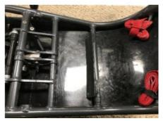
5. Slide the Repair Channel over the Seat Pivot.
