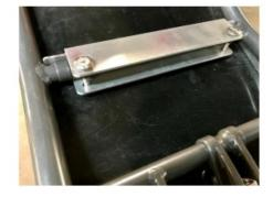
If you are having difficulty, inspect that the Seat Pivot Plate is flat and the rants are straight. They may have bent with a broken weld.
