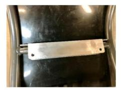
8. Check that the new 1/4-20 x 1 1/2" Sidewalk Bolts thread all the way through both sets of holes in the Repair Channel.
