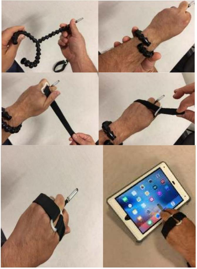
2. The Easy Flex Stylus is a flexible rod you can adjust by bending to fit your needs.
