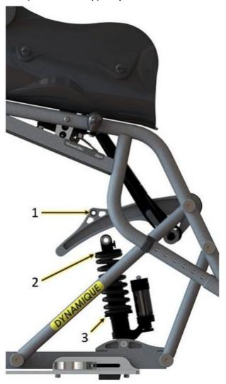
A 400lb spring is not a universal recommendation to suspension setup. When a significantly wrong spring rate is used it reduces the skier's ability to absorb the terrain and causes premature wear to you shock and ski.
