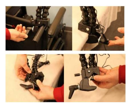
2. You can also remove one of the Easy Flex Dual Ultimate Switches from the clamp if only one switch is needed. To do this loosen the set knob on the clamp, then depress the spring loaded pin and lift up on the Flex arm to remove the switch from the clamp. See photos below.
