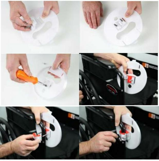
Option 2 is for mounting to a gooseneck mounting system with a  $\frac{1}{4}$ -20 threaded female socket. Attach your device's mounting tray to the adapter and secure with the two Phillips head screws. Thread the adapter with the  $\frac{1}{4}$ -20 screw into your gooseneck. Place your device into the mounting tray and press down to lock in place. See photos.
