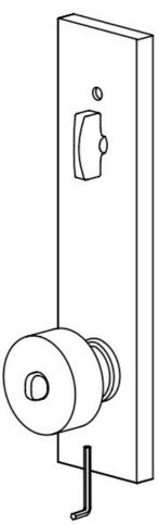
**STEP 2:** Unthread nut counterclockwise to remove from Interior Plate before installing on door.
