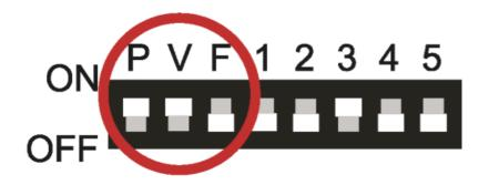
The PVF switches control the device's power supply, adjust the sounder volume and, if necessary, initiate flash only mode (sounder off).
