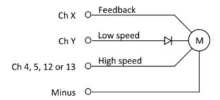
Any channel can be used for Ch X and Ch Y. Channel 4, 5, 12 or 13 is used as high speed channel. **Note:** The diode is never connected to channel 4, 5, 12 or 13.
