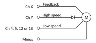
Any channel can be used for Ch X and Ch Y. Channel 4, 5, 12 or 13 is used as low speed channel. Note: The diode is never connected to channel 4, 5, 12 or 13.
