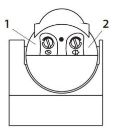
Infra-red motion sensors are used for automatic switching of lights in both indoor and outdoor areas. The sensor responds to the heat of persons moving in the detection area. On the intrusion of the detection field, a connected device is automatically switched on for a set period.
