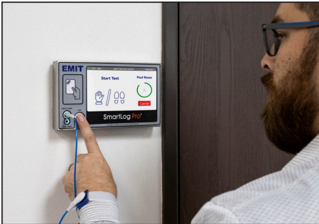
Figure 24. Performing a single-wire wrist strap test
