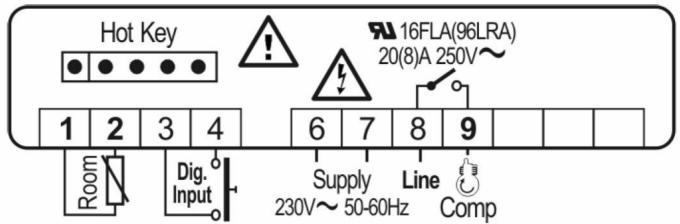
NOTE: in case of 110Vac model, connect power supply to terminals 6-7.
