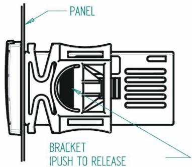
Instrument XR02CX shall be mounted on vertical panel, in a 29×71 mm hole, and fixed using the special bracket supplied. The temperature range allowed for correct operation is 0 to 60°C. Avoid places subject to strong vibrations, corrosive gases, excessive dirt or humidity. The same recommendations apply to probes. Let air circulate by the cooling holes.
