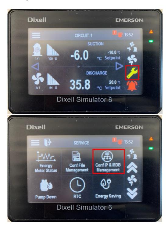
The default IP address of the controller is 192.168.0.250.
