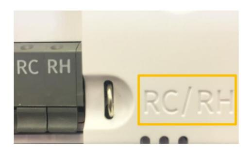
No jumpers are required when installing the Sensi Touch Smart Thermostat
