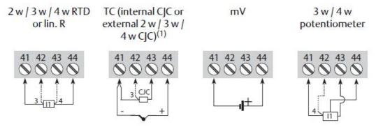
1. When using thermocouple input, the transmitter can be configured for either constant, internal or external CJC via a Pt100 or Ni100 sensor. This must be selected during device configuration.
