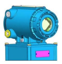
• Make sure endcap O-ring is installed.
