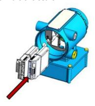
Install CPU module TB-1 and TB-2 and I/O module terminal connectors
