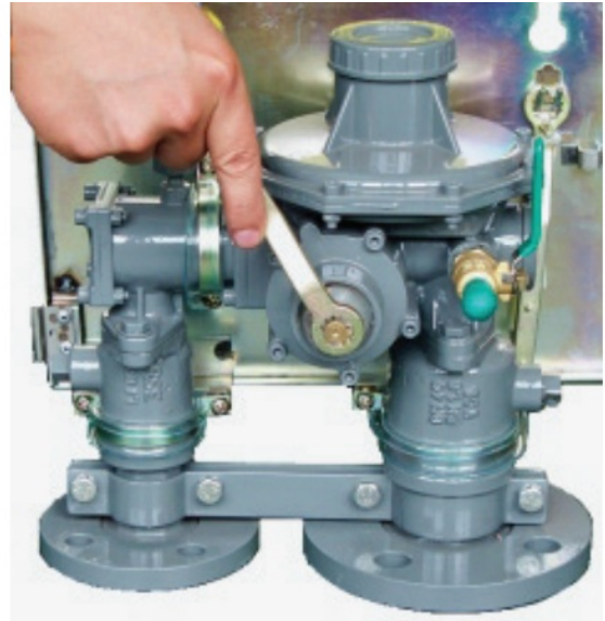
Figure 7. Slam-Shut Setting Adjustment
