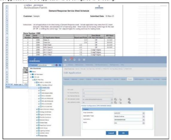
For AHU shedding, as in this example, select the Power tab, then select the Pointer Setup for the Pri Demand Shed and select the controller being configured, and then the application named Flexible Combiner, Demand Response and the output DO1. Next, set the Pri Demand Bump property to the specified number of degrees (5.00 in the screen above), as provided in the Shed Schedule form. Click OK to save the settings for both the Pointer Setup and Edit Configuration dialog boxes.
