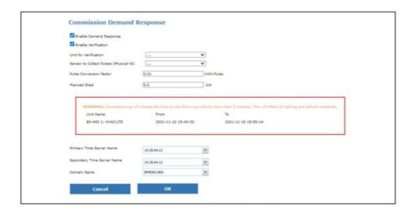
Verification and the unit and AI sensor/pulse meter to be used for verifying the shed events from the drop-down boxes. The Pulse Conversion Factor should be set to 0.001 kWh/pulse. If a sensor for the main meter pulses is not listed or defined, one will need to be created by the technician responsible for the programming of the E2. (Contact technical support for any questions).
