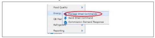
You can utilize this to quickly view the site shed time and find sites that failed to communicate and did not receive the command.
