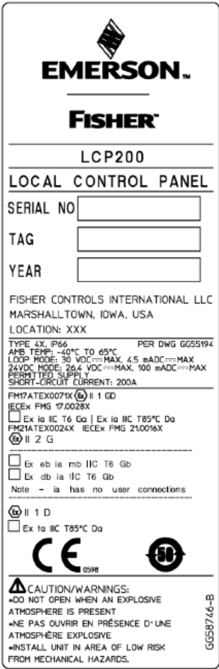
Figure 10. LCP200 ATEX/IECEX Nameplate, Explosion-proof, Group IIB
