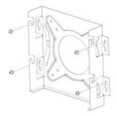
3. Mount the enclosure to the adapter fastened on the wall.
