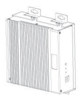
The above shown mounting direction is recommended for best efficiency of heat dissipation.
