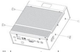
2. Install the mounting adapter to the wall, using the 4pcs M4x10mm screws.
