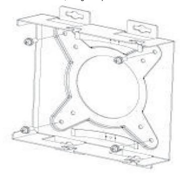
3. Mount the enclosure to the adapter fastened on the monitor.
