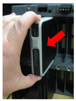
2. Press the new replacement module into the slot until it is properly seated.
