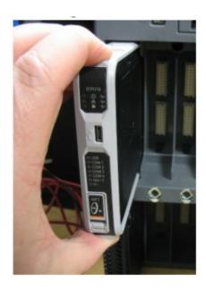
4. Press the new replacement module into slot 1 until it is properly seated.
