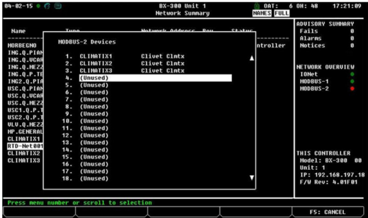
Figure 7 - MODBUS Device Address Selection
