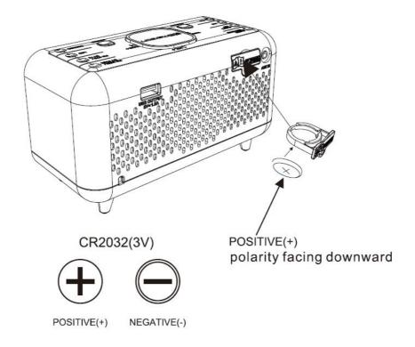
The lithium backup battery needs replacement when the LOW BATTERY indicator flashes, otherwise, the time and alarm settings will be lost/reset after a power outage.
