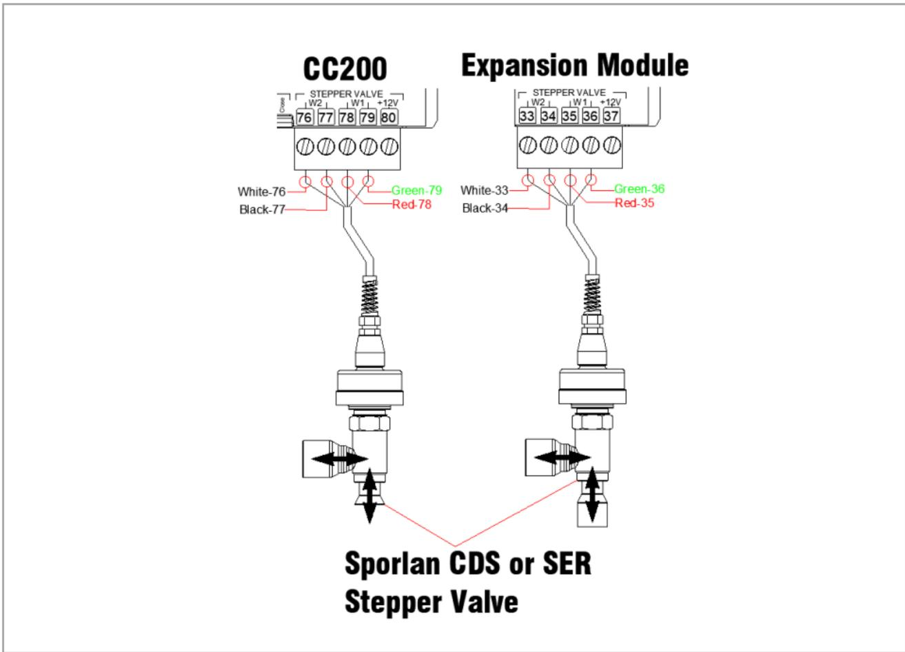
CC200 Expansion Module Wiring and Specifications
