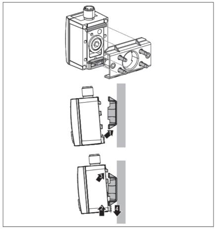
• Fig. 11: Mounting kit with mounted pressure sensor
