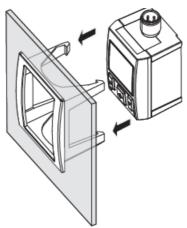
• Fig. 15: Attach the mounting kit at the lower mounting clip of the pressure sensor and let it catch
