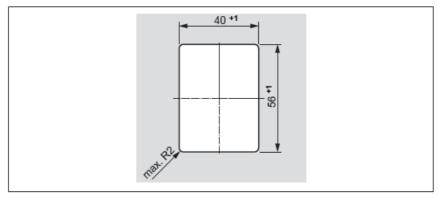
• Fig. 13: Insert the front frame in the cut-out
