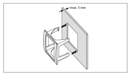
• Fig. 14: Push the pressure sensor onto the front frame
