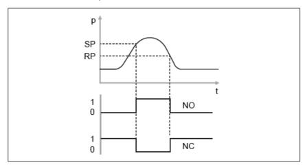
• Fig. 4: Hysteresis function in case of underpressure
