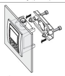
• Fig. 16: Fix in place and secure with mounting screws
