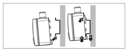
• Fig. 8: DIN rail with mounted pressure sensor
