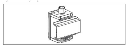
• Fig. 9: Fix the R412010405 mounting kit with two screws
