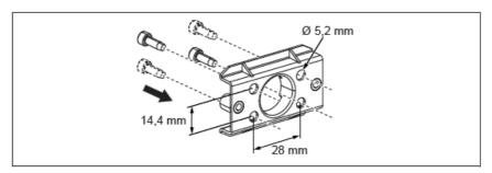
• Fig. 10: Center the pressure sensor on the mounting kit and hook it in place
