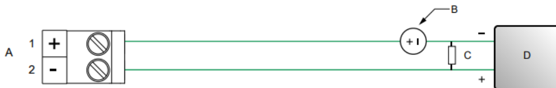
Figure 2-1: Channel A mA/HART output wiring (externally powered)
