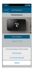
**Pro Tip:** If you are DIYing your installation, always choose Not Mounted to make sure your thermostat is wired and configured correctly.
